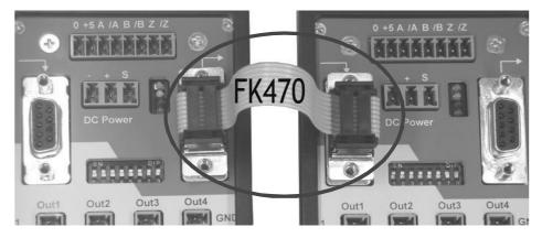
Cascading lines use the same common GND potential as the power supply of the unit. This however does not mean any disadvantage in terms of galvanic isolation etc. since cascading units are always mounted alongside and are also supplied from the same power source.
